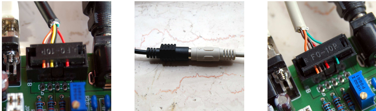
Figure 22: Different connections of the Fortuna U2-PS/2 to the evaluation board.
