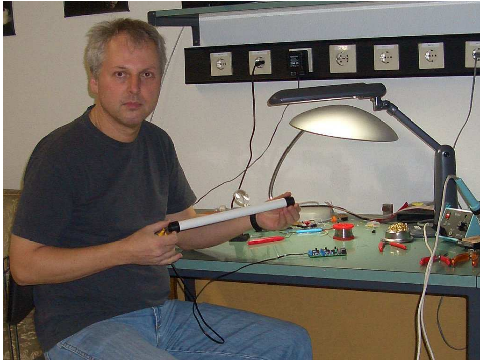
Figure 7: A 35 cm ferrite rod antenna in my hands.
